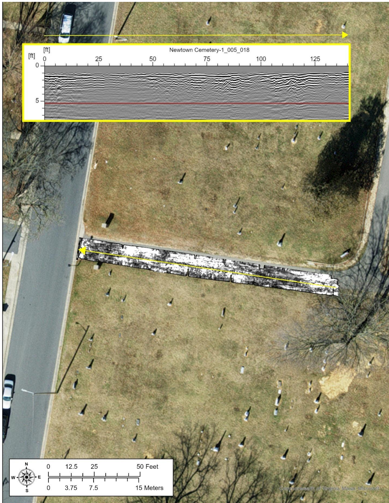
Figure 4.7. The Effinger Street MALA HDR survey and representative reflectance profile (inset).
